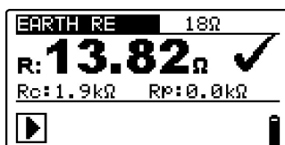
Figure 5.32: Example of earth resistance measurement result
